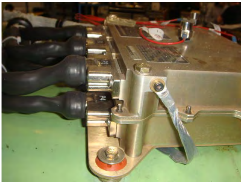
Figure 76-17: ECU Bonding Jumper Installation.
