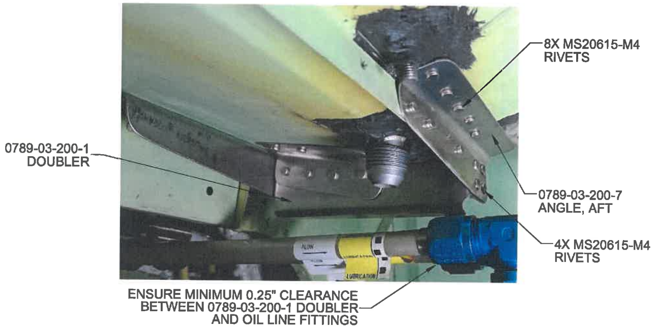
FIGURE 2: REPAIR AREA LOOKING OUTBOARD UNDER FIREWALL PAN
