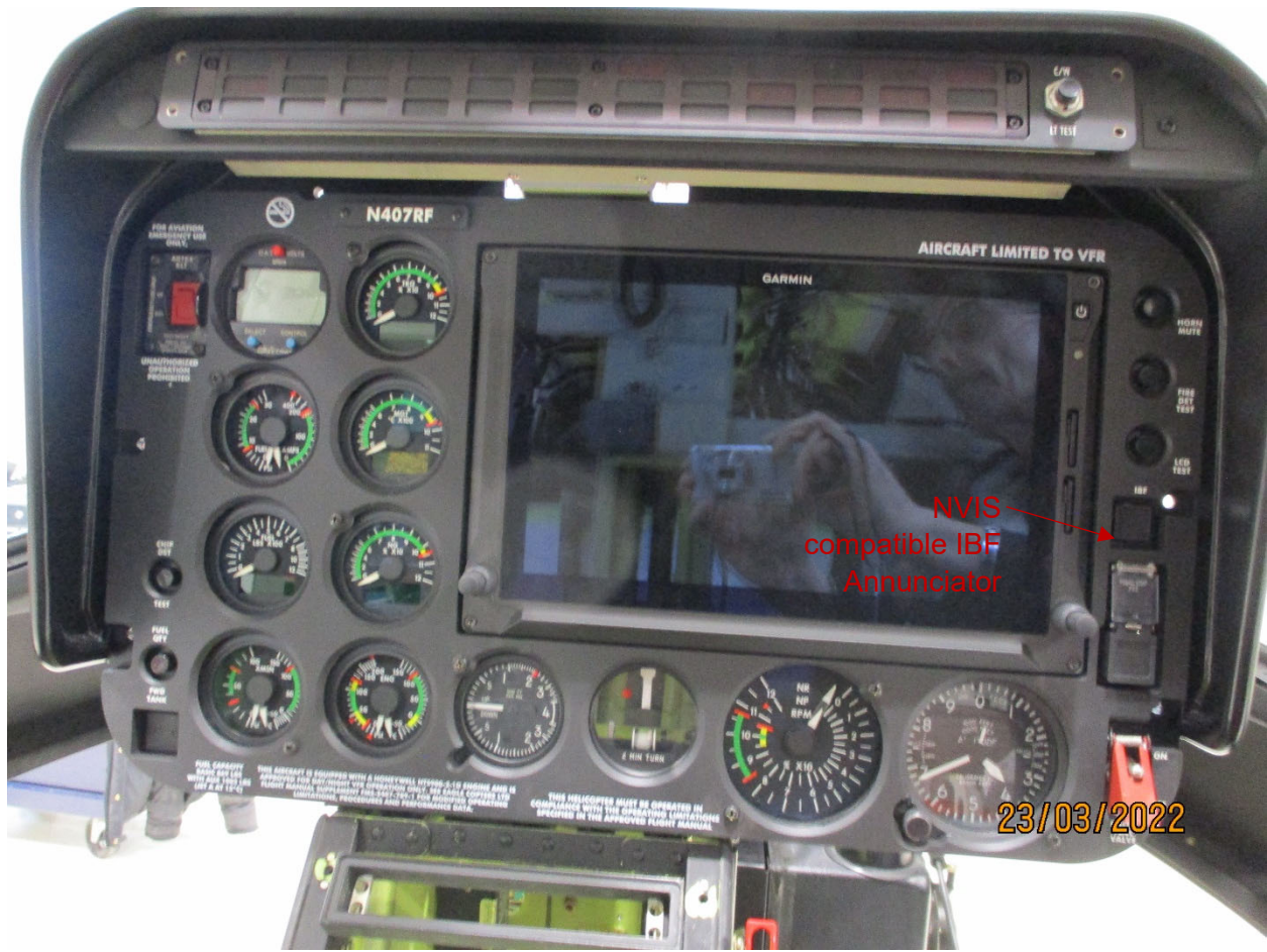
Figure 4 -015 Kit Installation IBF Annunciator (Below LCD test switch on RH side)
