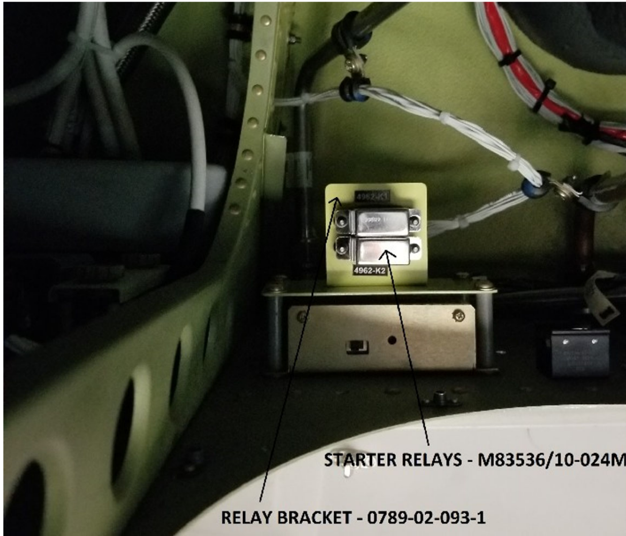
Figure 13 - POST TB - STARTER RELAY AND BRACKET (-011 INSTALLATION)
