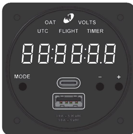
Figure 6 – Display Test (6420093-5 unit shown with USB-C connector)
